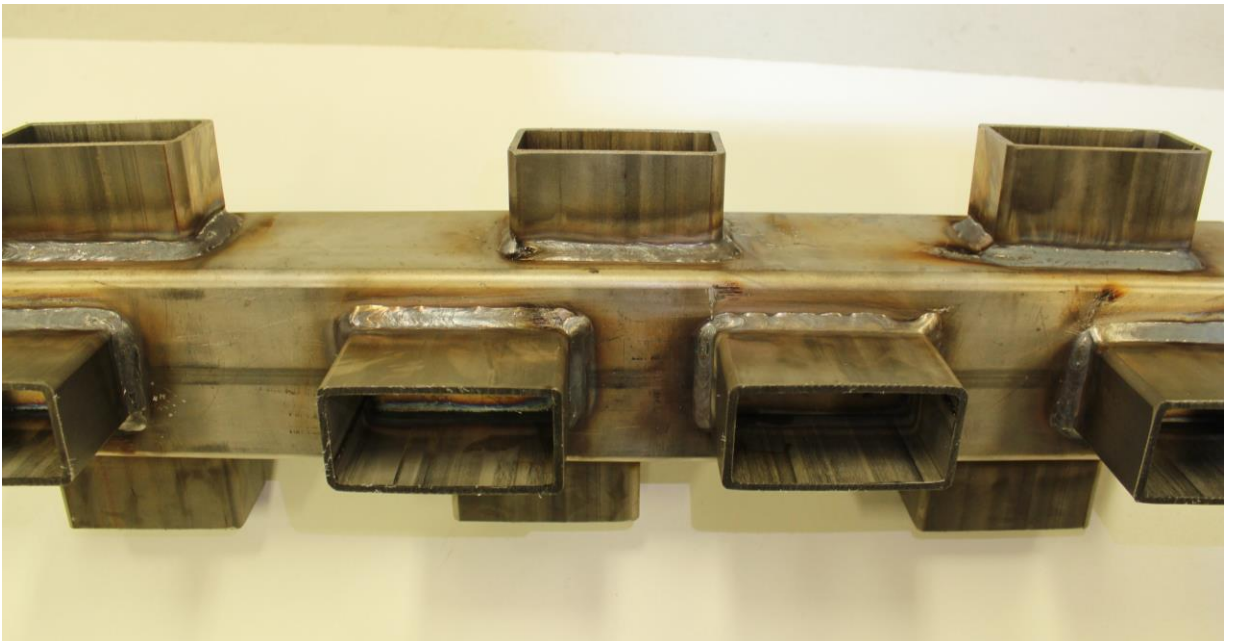
Sample A/B: Image A.5 – before pickling
