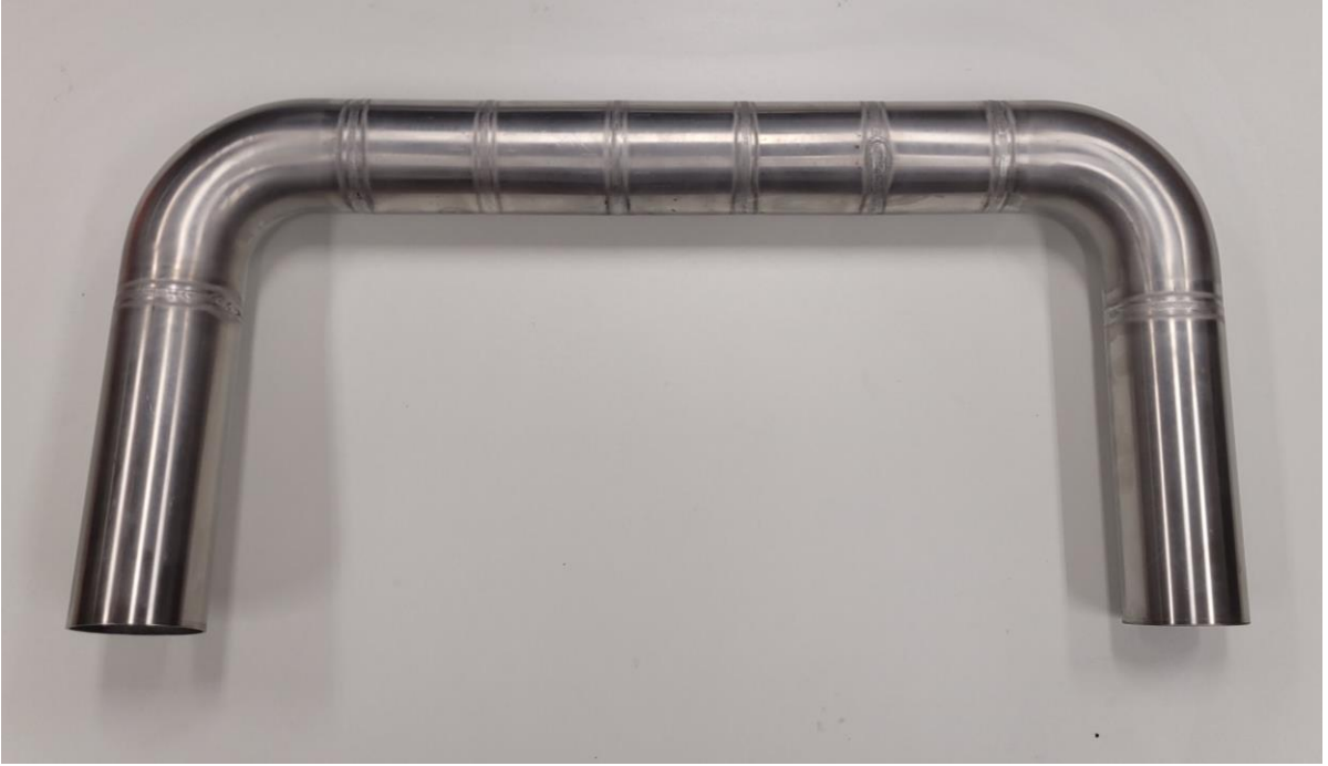
Sample C: Image C.2 – after pickling
