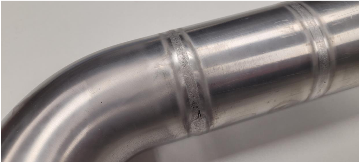
Sample C: Image C.4 – after pickling
