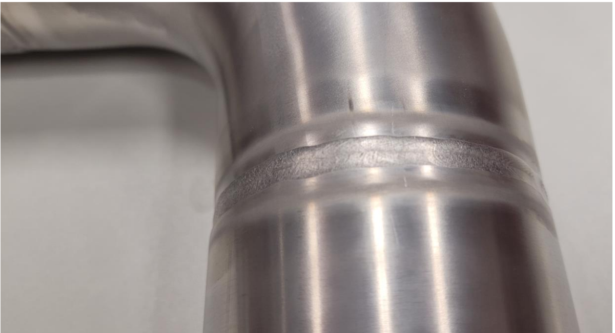
Sample C: Image C.3 – after pickling
