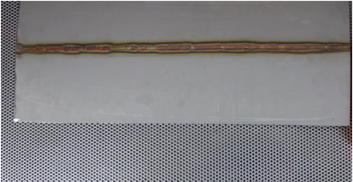
Sample E: Image E.1 – before pickling
