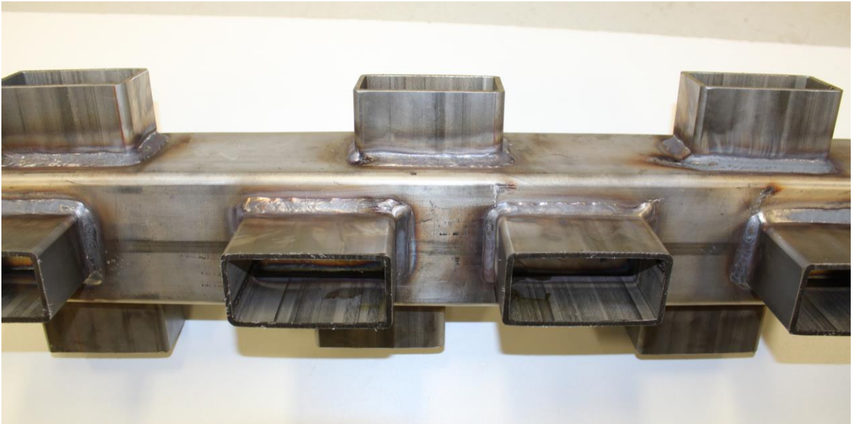
Sample A/B: Image A.4 – before pickling
