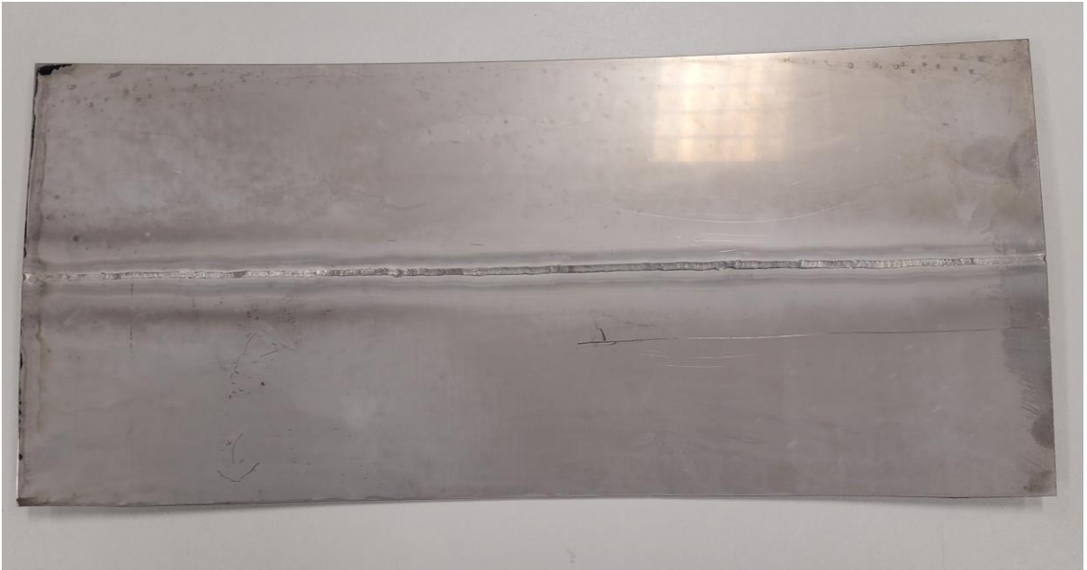
Sample E: Image E.2 – after pickling
