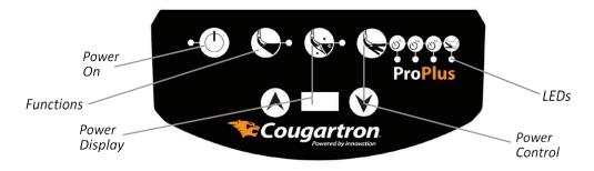
The Power is adjusted by the 2 buttons either side of the small screen. The power is adjustable in increments of 5 amps from 05 to 50. The screen displays how many amps the machine is running on. The Power setting switch is used to adjust the amount of voltage applied to the brush, and therefore how fast the Cougartron ProPlus cleans.
