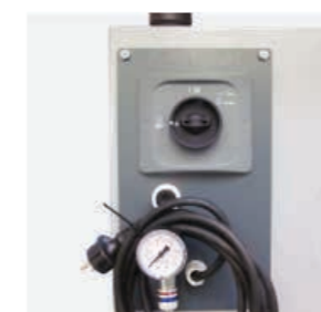
Motor protection and compressed-air Equipped with integrated motor protection and compressed-air connection.
